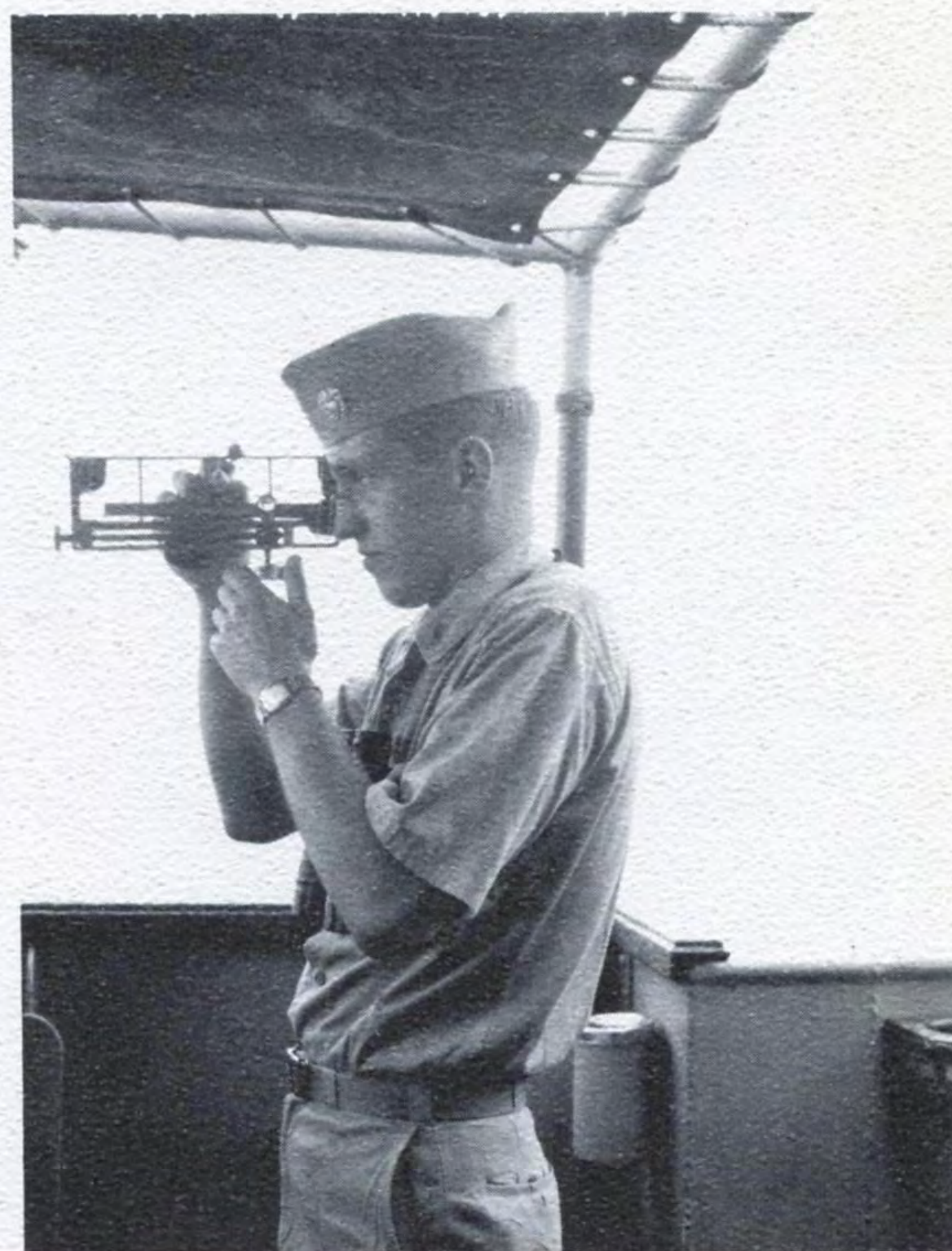
ENS Marlowe, Assistant Anti-Submarine Warfare Officer, determines the range to another ship by using a stadimeter.
